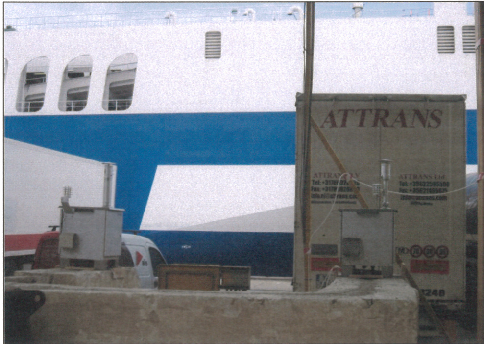
Figure 2: Positioning of two instruments: one SKYPOST for PM 10 and the other for PM 2.5
