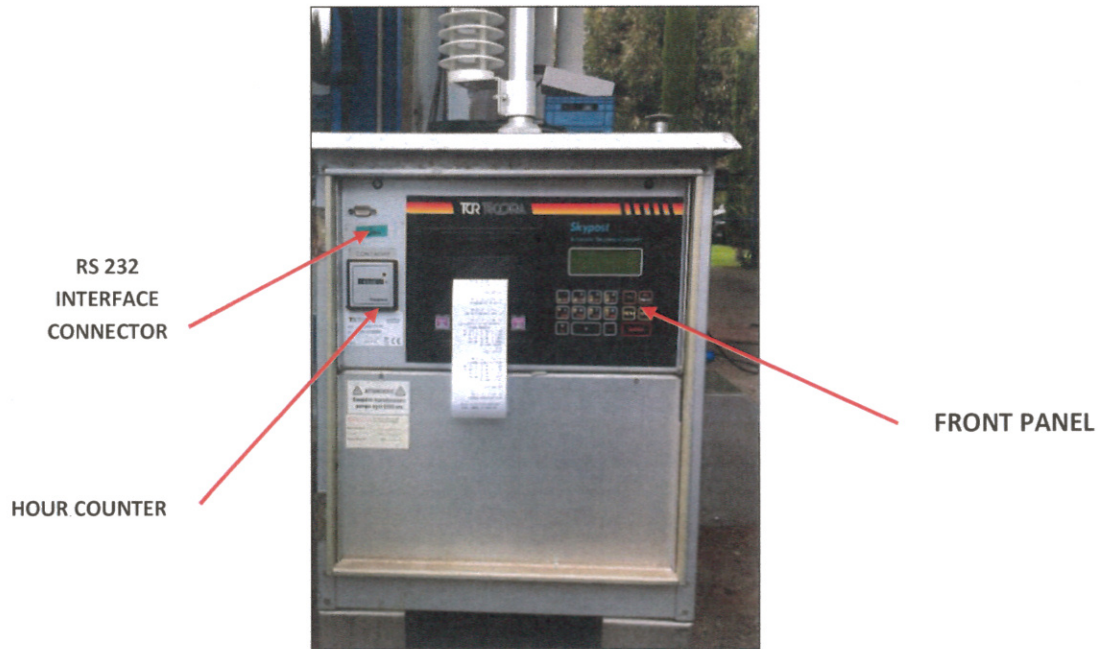
Figure 11: SKYPOST PM HV – backside detail
