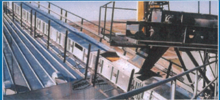
Able to convey most grains at angles of up to 25 degrees (18-degree incline shown). For steeper angles, contact Brock for recommendations.
