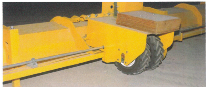
Sweep Drive with Foam-Filled Dual Wheels
