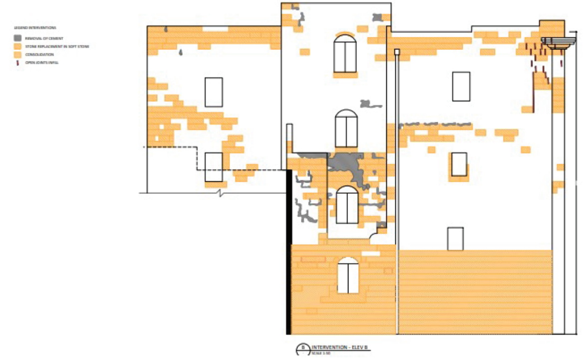
Restoration of Façade, Mapping of Materials – Cospicua
