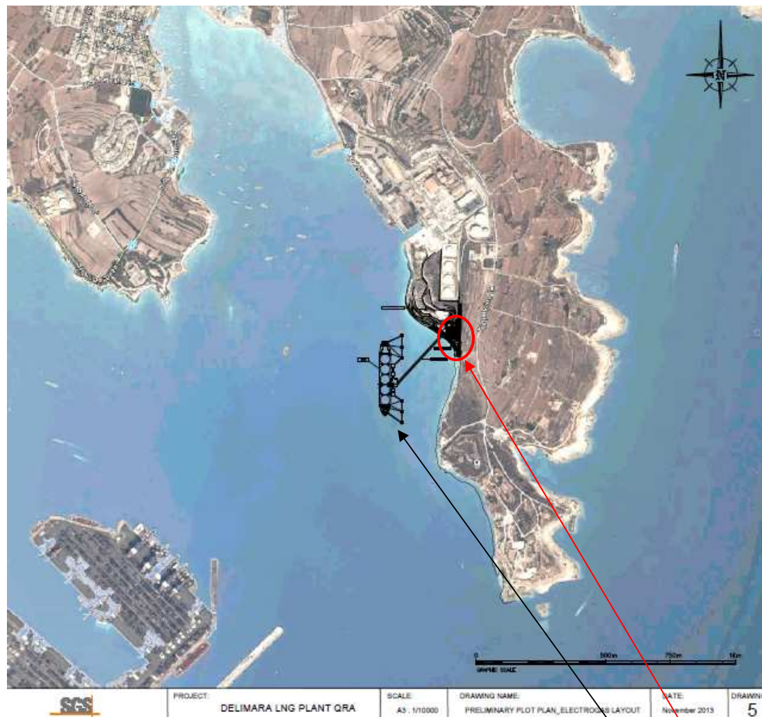
Figure 6.2: The proposed location of the main units of the LNG terminal : FSU and RU [10]
