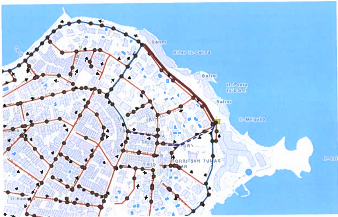
Figure 20 Proposal for new rising main to cater for additional load (Source: WSC)
